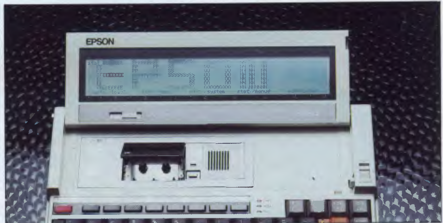
A ratchet mechanism allows the display to be set to various angles
